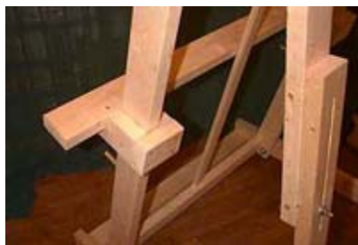
fig 3: shelf support detail (rear)
